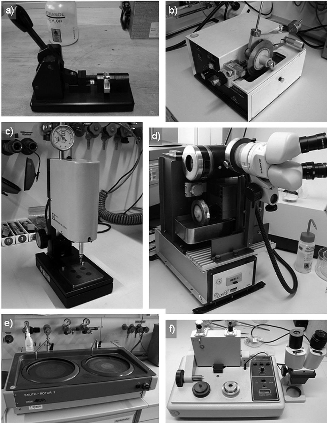
Fig. 7.2: Several examples for preliminary preparation tools used in TEM specimen preparation: (a) punching tool, (b) wheel saw, (c) ultrasonic disk cutter, (d) wire saw, (e) rotary grinder/polisher, (f) dimple grinder.
