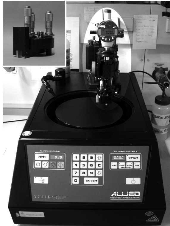
Fig. 7.10: Automated tripod polishing machine for precise control of specimen thickness, wedge angle and applied load. A simpler hand-held version is shown in the upper inset.
