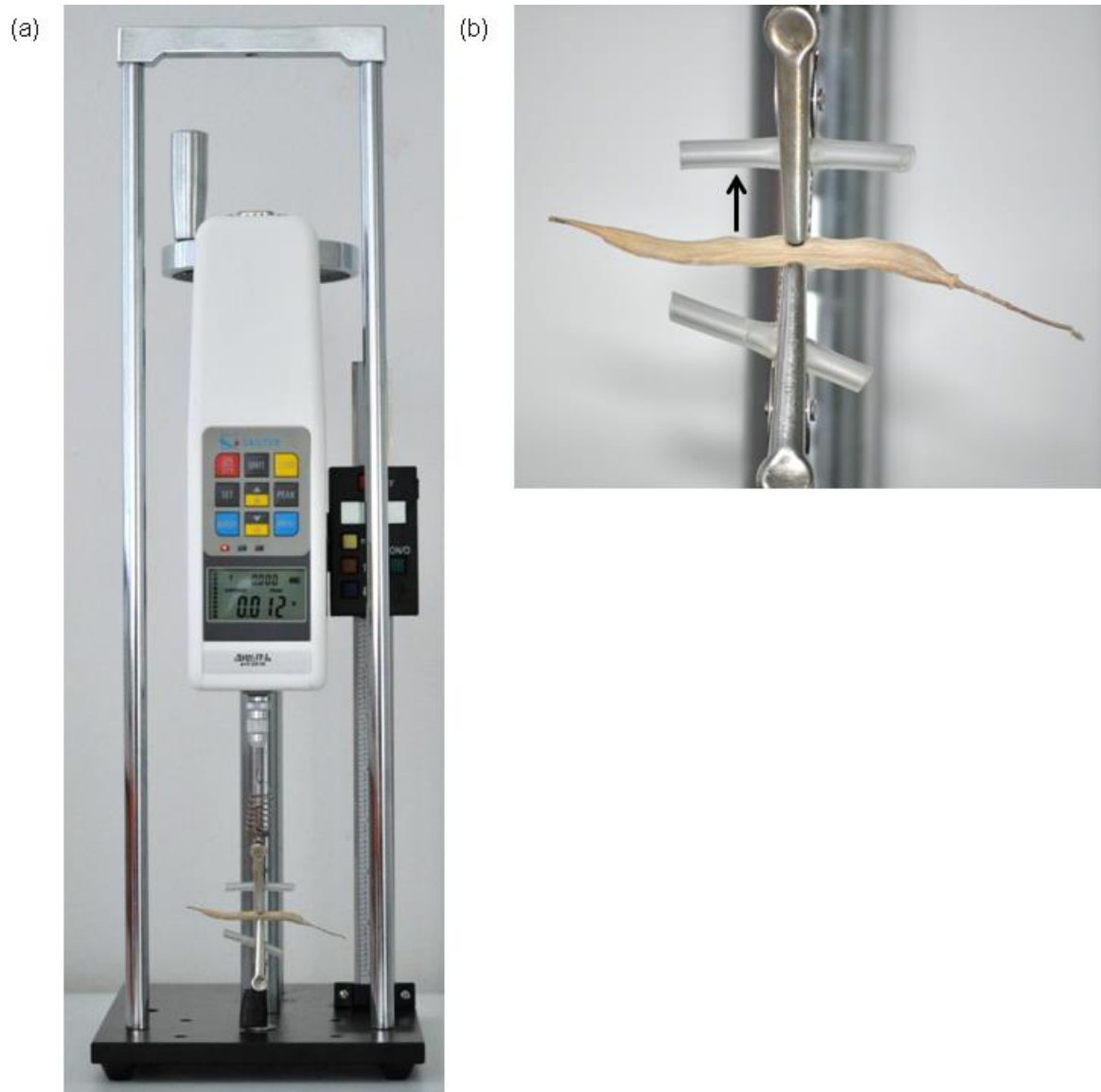
Figure S9. Experimental set-up of the tensile force measurement. (a) The Newton meter test-stand is loaded with a silique. (b) Close-up of a silique fixated with two alligator clamps. Tensile force will be applied in the direction of the black arrow.
