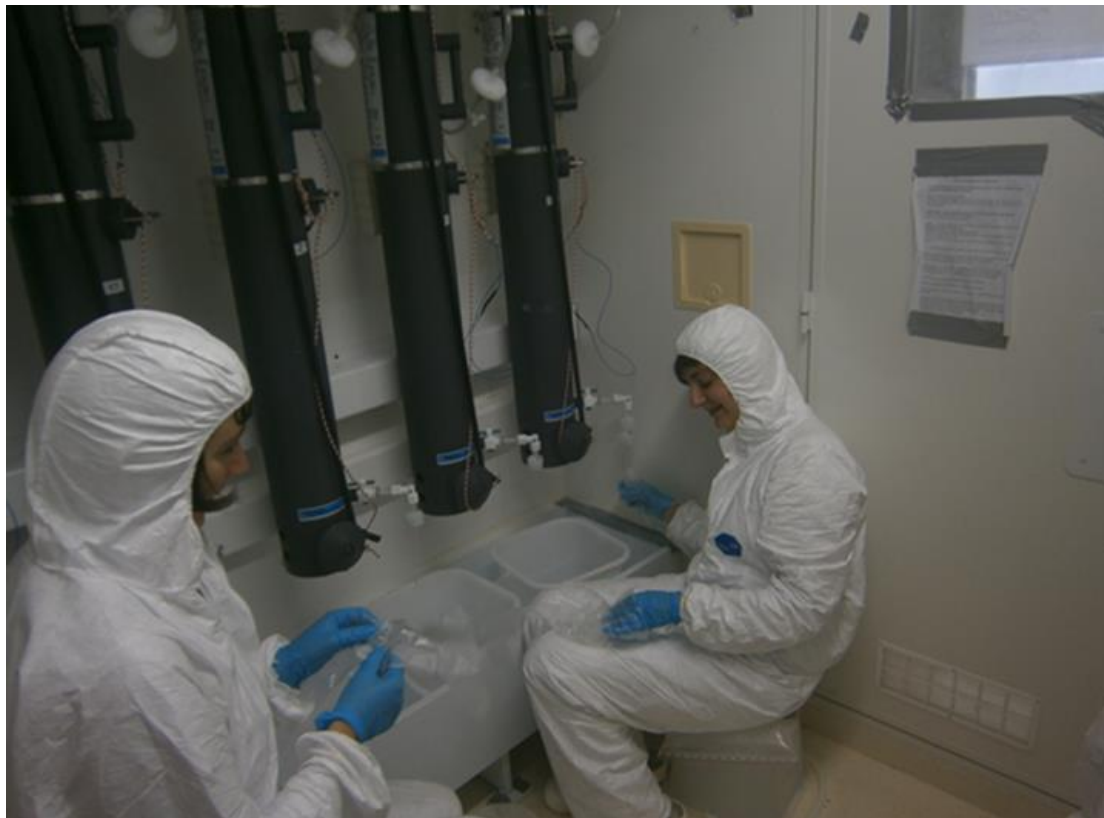
Figure 2.3: GO-FLO bottles attached to the wall of the clean container and ready to be sampled.
