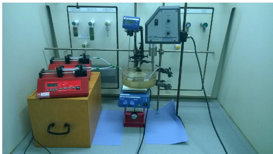
Figure S3.1. Photograph of the two syringe pump configuration of the flow reactor including the ultrasonic probe (centre).
