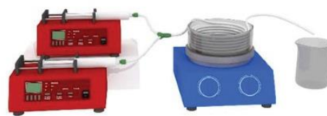
Fig. 1 Schematic of the flow reactor in a two pump configuration, showing the hotplate and oil bath in which the coil of PTFE tube forming the reactor is immersed.
