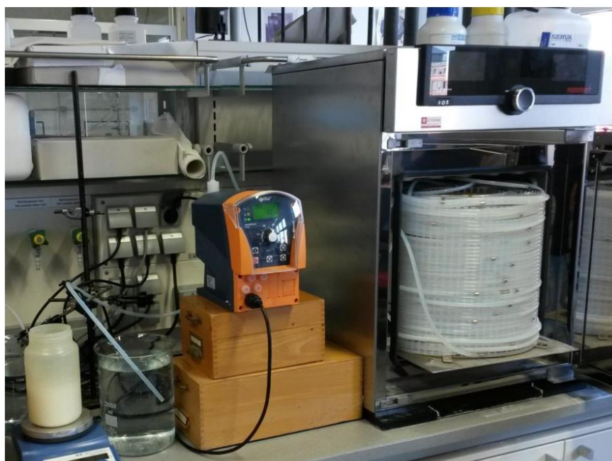
Figure S11: Set up of the flow reactor.
