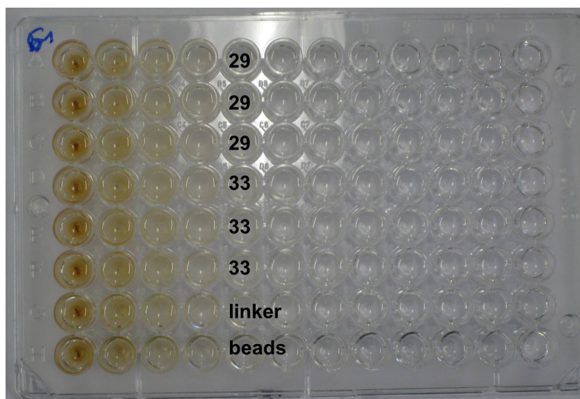
Figure 8.25. Agglutination of magnetic PEG beads in a serial dilution decorated with mannosides 29 or 33 ; using type 1-fimbriated E. coli bacteria. The depicted figures are representative examples from at least three independent experiments. Carboxylic acid beads blocked with ethanolamine and beads decorated with the Fmoc-deprotected linker molecule were tested simultaneously on each plate.
