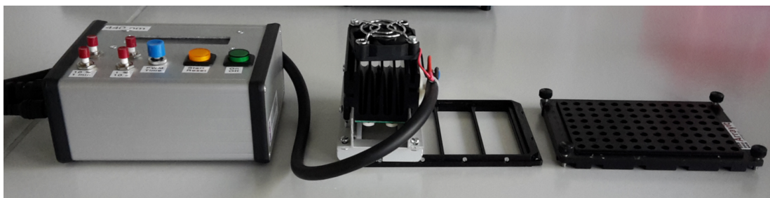
Figure 7.3.3: Setup for irradiation experiments. Glass slides were fixed in the microplate microarray cassette (Arrayit corporation, CA, USA). LEDs were arranged to exposure 1 quarter of the plate uniformly. Distance between glass slides and LED was 1 cm. Top of the plate (right) was added for adhesion of bacteria and the fluorescence readout in a microplate reader.
