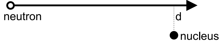
Figure 1.3: Neutron trajectory in the vicinity of the nucleus. d is the shortest distance between neutron and nucleus. It can be shown, that d must be quantized and that only neutrons without angular momentum ( l = 0 ) can interact with the nucleus.
