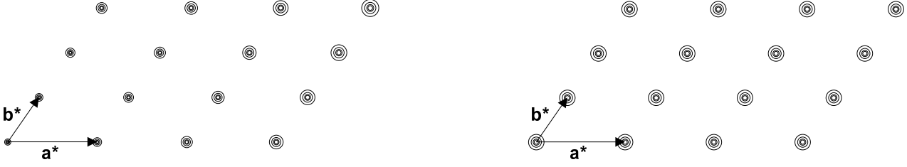
Figure 3.6: Effect of strain (left) and particle size (right) broadening on reciprocal lattice points (after Von Dreele, 1989).
