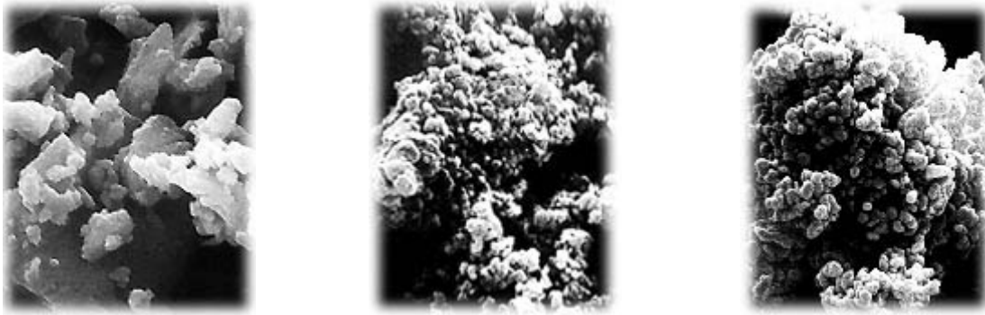
Figure 3.18: TEM picture of dead, hard and light burned MgO [from left]. Clearly visible is the reduced particle size leading to larger surfaces areas [MMM].
