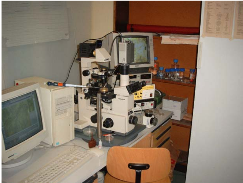
Figure 2.1: Experimental device setup for video microscopy. To the left, the recording computer, in the middle of the figure, the microscope with video mount, and to the right, the video recording. (scale: height of computer is 38 cm)
