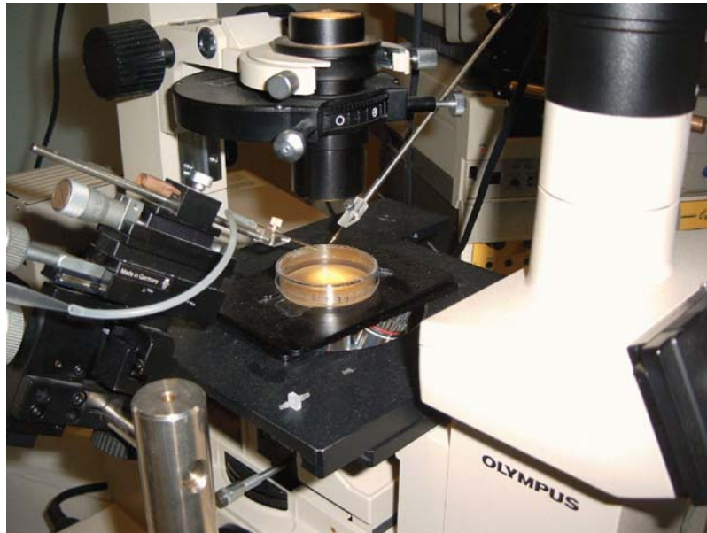
Figure 2.2: View of the microscope of figure 2.1 with a petri dish in the center ( \phi 5.5 cm) and a micromanipulator to the left.
