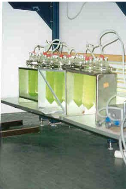
Figure 5.1. Typical set-up of a growth experiment. Eight growth vessels were installed in front of a light tube and bubbled with air.
