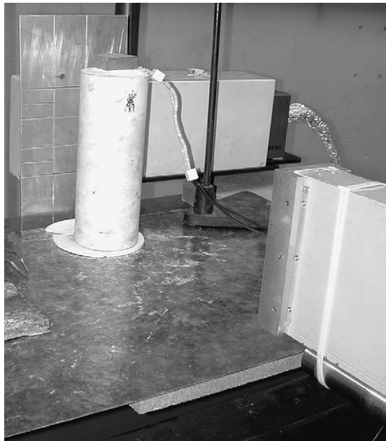
Fig. 1. Experimental set-up. The end of the neutron guide is shown at the right. The neutron converter, scintillator and video camera are enclosed in the rectangular box behind the tube furnace. The height of the furnace is 300 mm.
