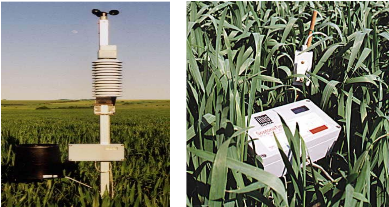
Abbildung 7: Wetterstation Modell Thies/Weihofen und Septoria-Timer Modell Thies CLIMA (THIESCLIMA, 2001; NUM. MATH. UNI-GOETTINGEN, 2001)
