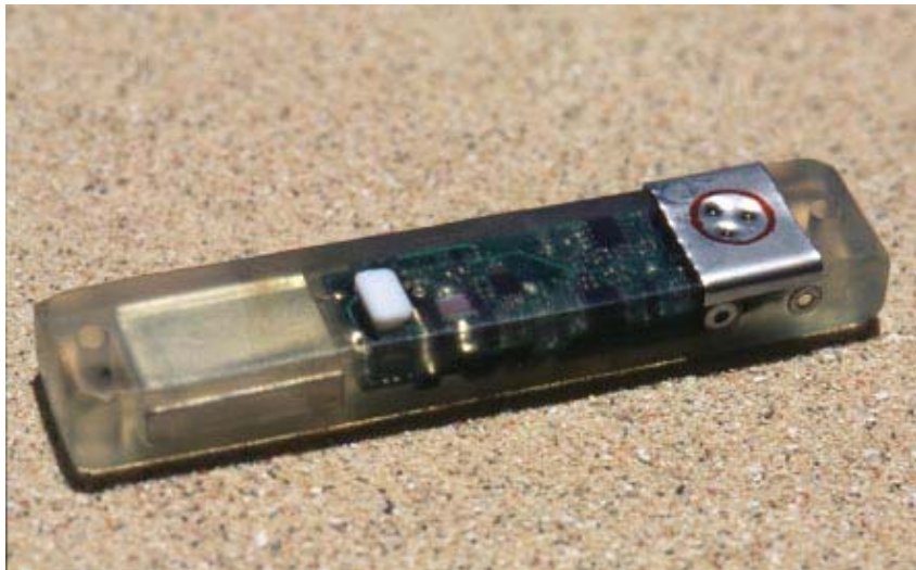
Fig. 13: The Mk7 (Wildlife Computers, Redmont, USA) used for the long-term study.
