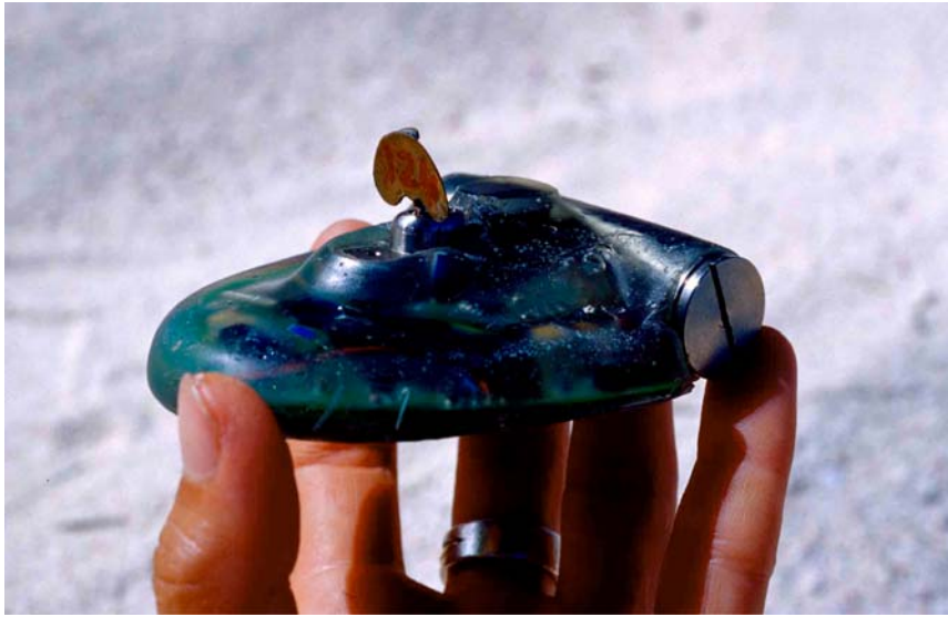
Fig. 7: The data-logger DK602 with miniature paddle for velocity readings.
