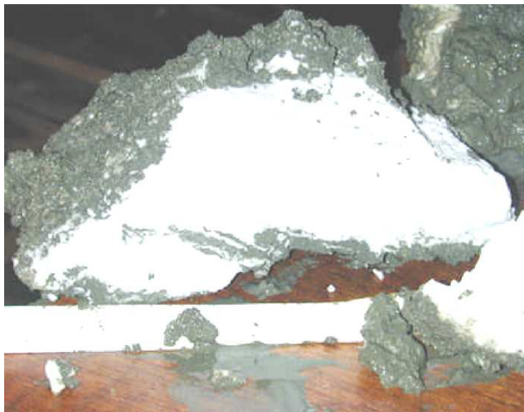
Figure 2.10: Natural methane hydrate sample collected by GEOMAR from the Hydrate Ridge in the north Pacific Ocean. The white methane hydrate is covered with a layer of sediment.
