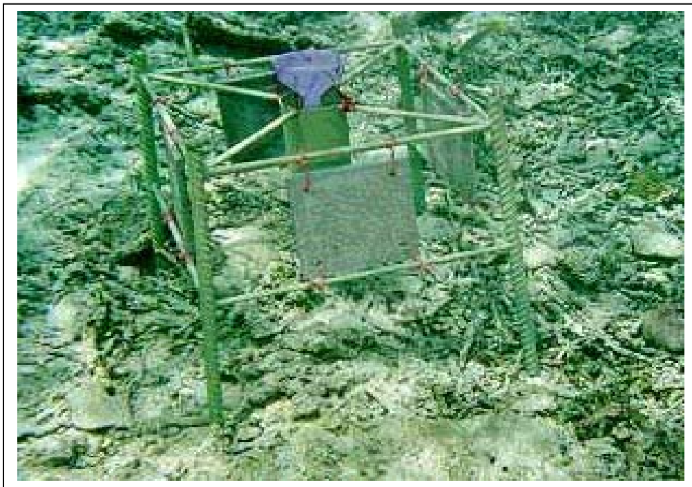
Plate 2.3: Metal racks holding the concrete substrates attached by wire and a small sediment trap in the center
