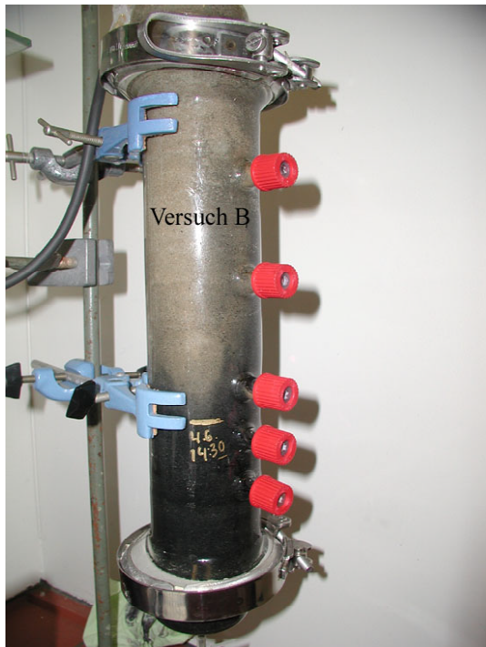
Figure 4-1: Snapshot of reaction column S3 (natural aquifer sand) showing the black, reduced section in the lower part and the untreated section in the upper part 24 h after the experiment began.
