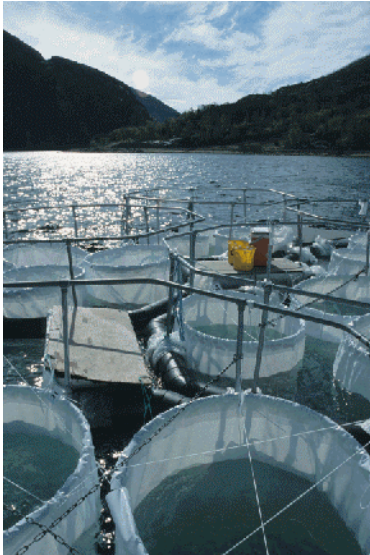
Picture 2-1: Enclosure bag set-up in Hopavågen fjord.
