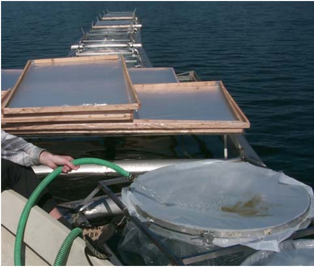
Picture 1-1: Filling of enclosure bags by screening Schöhsee water through a 55 \mu m gauze in order to remove zooplankton. Covers of enclosures are shown mid picture.
