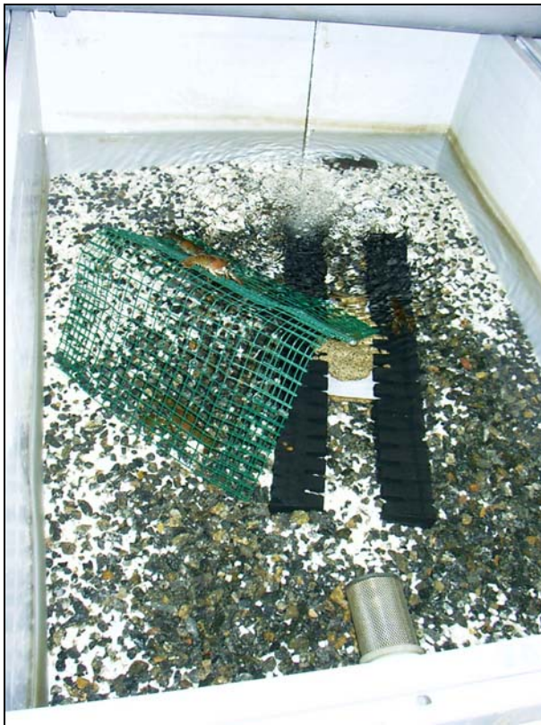
Picture 3 (left): Photography showing one of the tanks (0,6m x 0.8m) in the experimental system. A substrate from gravel was provided and shelters were given in excess (40 shelters for 20 animals).
