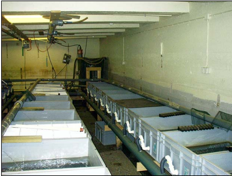
Picture 2: View of the experimental tank system as it was used for this study. The system was artificially illuminated (18L:6D photoperiod) and temperature was kept within a range of 17.5 to 19°C.
