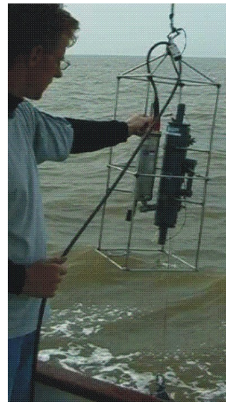
(c) Deployment of CTD from the right amidships of the vessel
