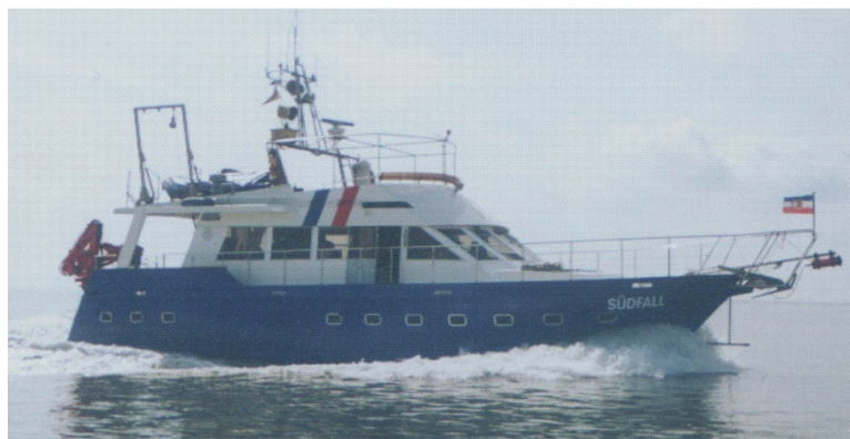
(a) Research vessel Südfall; ADCP mounted in the bow of the vessel is faced down during deployment; CTD is deployed from a winch in the right amidships of the vessel
