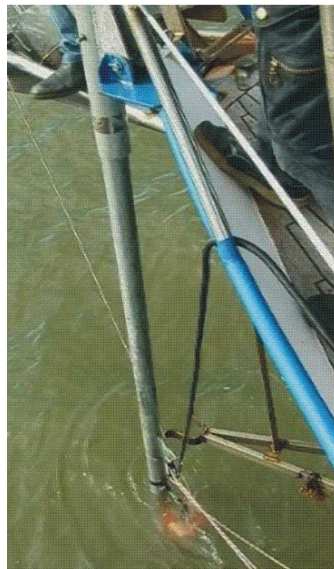
(b) Deployment of ADCP from the bow of the vessel
