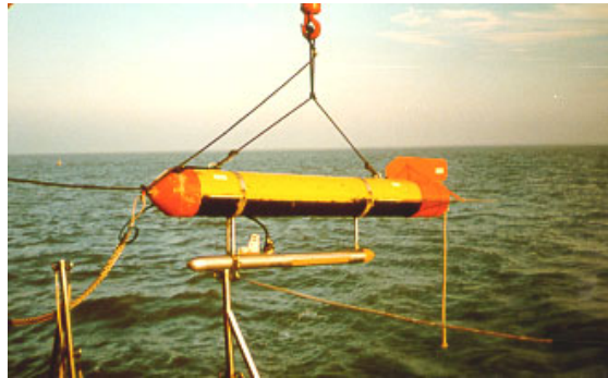
Figure 3.6: Klein 595 side scan sonar used to map the bottom of channels
