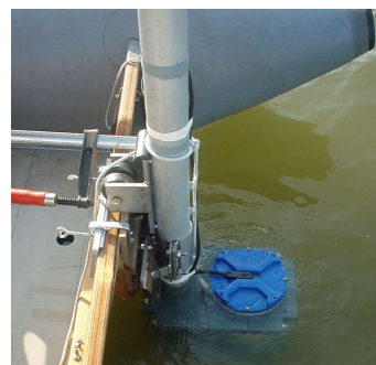
b) ADCP attached to the rubber boat
