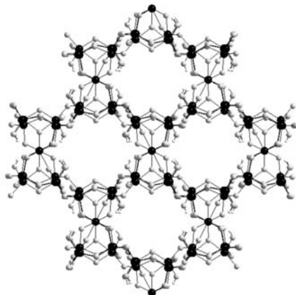
Fig. 3. The Ge 9 (OH) 4 O 18 framework with view along the [101] direction (the [1,2-DAPH 2 ] 2+ and water guest molecules are omitted for clarity).
