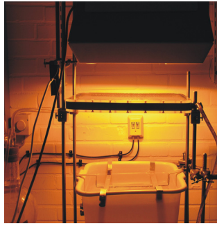
Figure 3.1 Experimental arrangement for applying high-light conditions of 800 \mu\text{mol m}^{-2}\text{s}^{-1} using SON-T Agro 400 lamp (Phillips, Hamburg, Germany).
