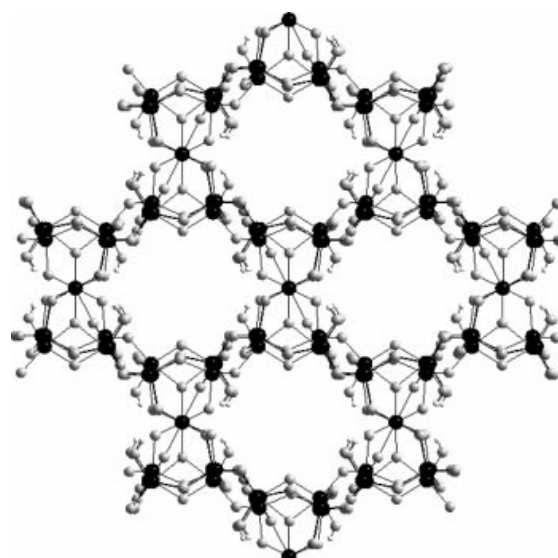
Fig. 1 The \text{Ge}_9(\text{OH})_4\text{O}_{18} framework of (1,2\text{-DAPH}_2)_2\text{Ge}_9(\text{OH})_4\text{O}_{18} \cdot 2\text{H}_2\text{O} with view along the [101] direction. Black spheres: Ge; grey spheres: O. The [1,2\text{-DAPH}_2]^{2+} and water molecules are omitted for clarity.
