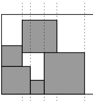
Figure 1.2: A sliced structure in a tight packing.
