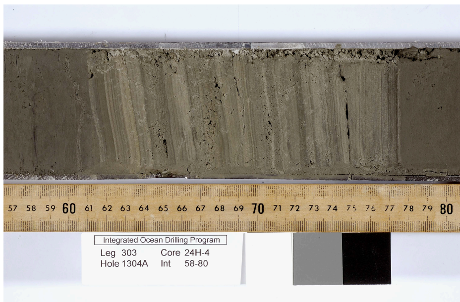
Fig. 2. Site 1304. Example of laminated diatom ooze in core split with saw showing the fine laminae characteristic of these sediments (Interval 1304A-24H-4, 59-80 cm).
