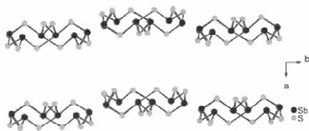
Fig. 5 Arrangement of the [\text{Sb}_9\text{S}_{15}]^{3-} anion in (\text{C}_7\text{N}_2\text{H}_{13}^+)_3\text{Sb}_9\text{S}_{15} (II) showing the large inter-chain separation along [100].
