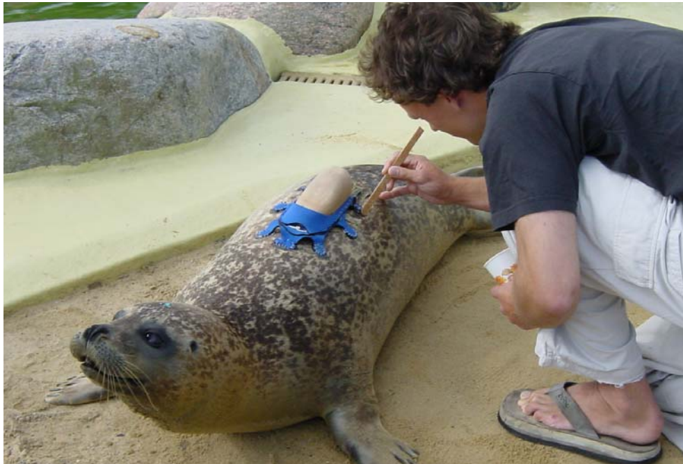
Figure 18. Attachment trial of a prototype neoprene base with device dummy on a captive harbour seal at the Seal Centre in Friedrichskoog.
