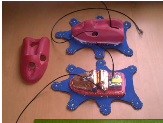
Figure 16. Package without release mechanism used during the spring deployments on harbour seals.
