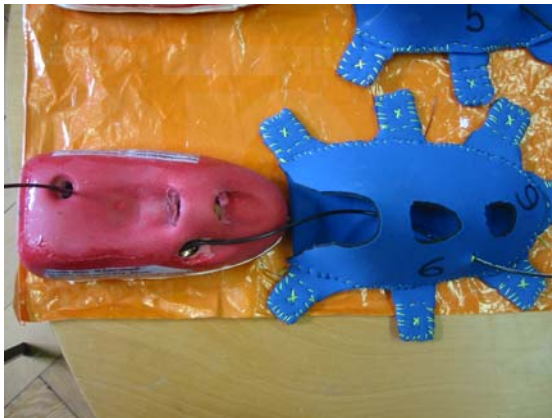
Figure 15. The neoprene base to which the flotation body is attached. The protruding legs are stuck to the seal's fur at their ends, the contact being enhanced by grids sewn to the material.
