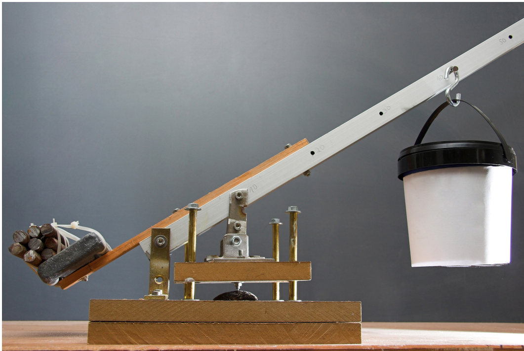
Figure 4: "Shell cracker", device for assessment of shell stability.
