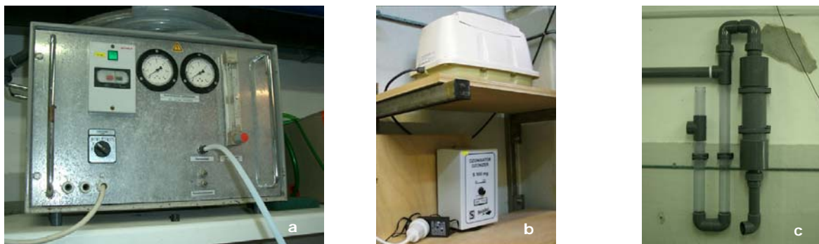
Fig. 10. Ozone generators used in this study: (a) laboratory 1 to 4 g*h -1 ozone generator (prototype); (b) 500 mg*h -1 ozone generator model S 500; and (c) air rest-ozone-killer.
