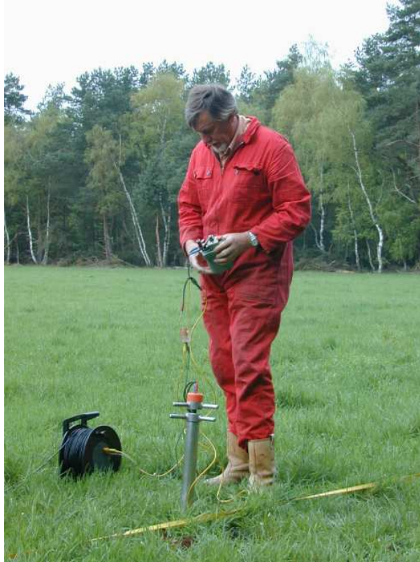
Figure 2.3: Mr. Druivenga from the GGA operating the Sissy (Seismic Impulse Source System) at Neuwarmbüchen.
