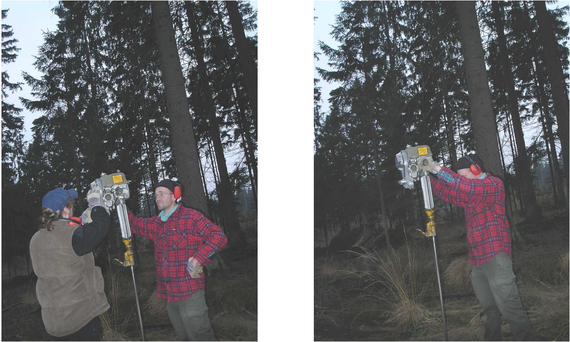
Figure 2.16: Percussion drill “Wacker” in use in the Segeberg Forest. Left: While starting, right: while drilling.
