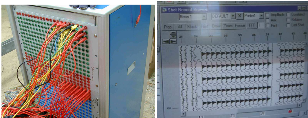
Figure 4.35: Left: All 1439 electrodes can be addressed at this control box. Right: Problems arise due to strong anthropogenic 50 Hz noise (screen shot of the Bison seismograph monitor during seismoelectric measurements at the GeoModel).
