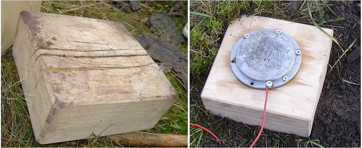
Figure 2.6: Metal disc screwed onto a wooden block. Left: Backside of the prototype which turned out to be too thin (10 cm) for the strong mechanic strains. Right: Successor model after some hundred hammer blows. Two out of six screws have already loosened. The red trigger cable used for the short-circuit trigger is screwed to the metal plate.
