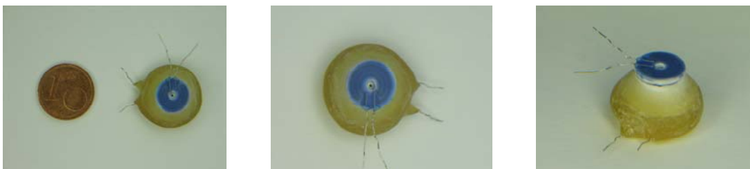
Figure 7.11: Photographs of top and side view of sensor C-4 with the heating element on top.
