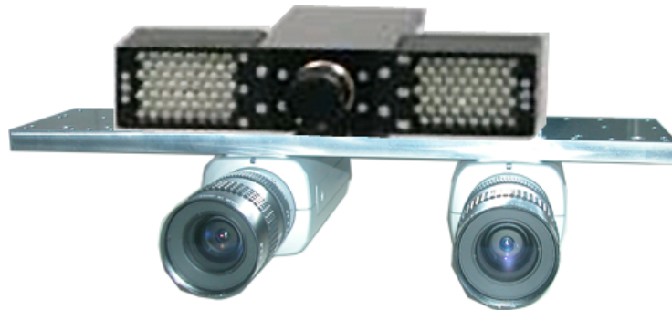
Figure 4.33: Setup used for the arm tracking. PMD camera on the top with IR-LEDs next to it.
