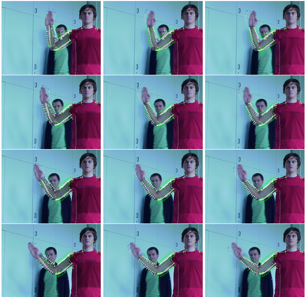
Figure 4.38: Silhouette correspondences are accurate though the background is very dynamic. Each row shows the iterations for one frame. Frames 40-43
