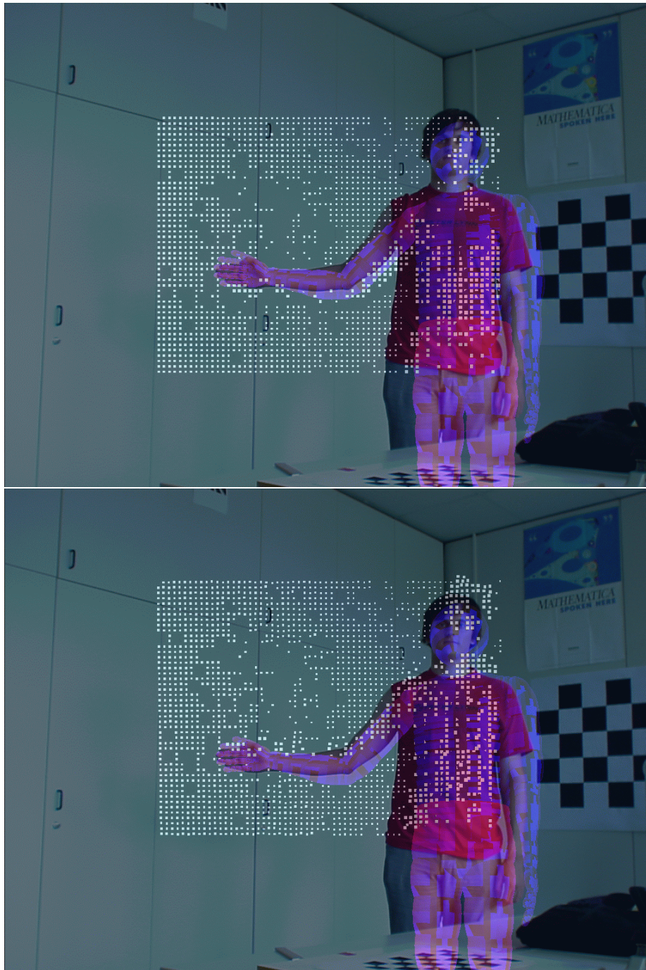
Figure 4.37: Calibration results: Depth points from PMD-camera projected into standard-camera image. Top: Same external parameters. Bottom: Applied calibration result.
