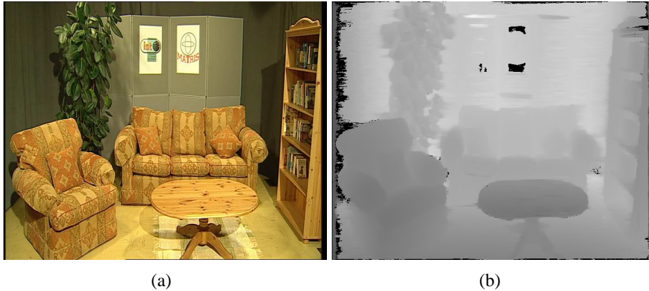
Figure 6.3: One original view from the Studio data set and the corresponding depth map.
