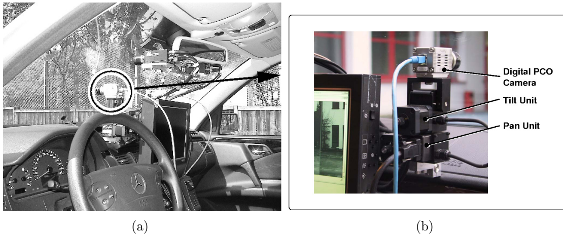
Figure 5.32: The UTA (Urban Traffic Assistant) demonstrator from Daimler Chrysler AG (a). Only one of the two PTU mounted cameras is used in this work. A closeup view of the pan-tilt unit mounted camera (b) (courtesy of S. Gehrig).
