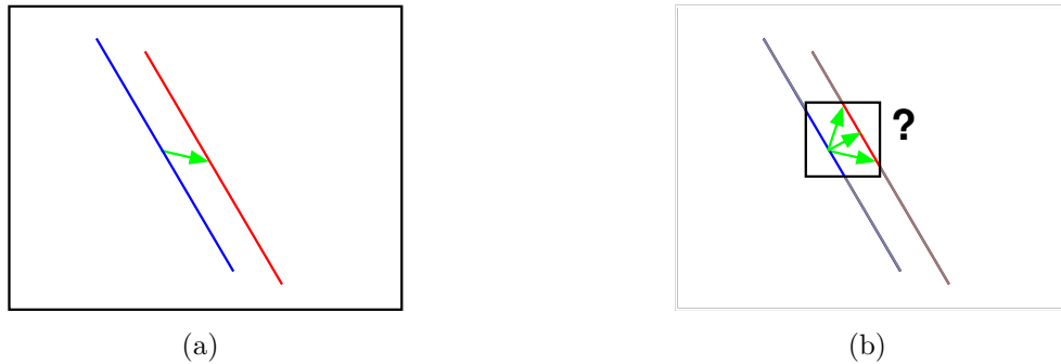
Figure 4.2: Visualisation of the aperture problem: Computation of the displacement vector of a 2D-line segment. The line is drawn in blue at time t and in red at time t + dt . (a) If the complete line including the endpoints is used, a human can easily guess the displacement vector. (b) If however only a small support window (black) is used when computing the displacement, a unique solution cannot be determined.
