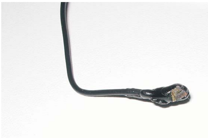
Figure 5.24: Picture of a \text{TaS}_2 sample connected by a copper wire and covered by apiezon wax, used for cyclic voltammetry experiments.
