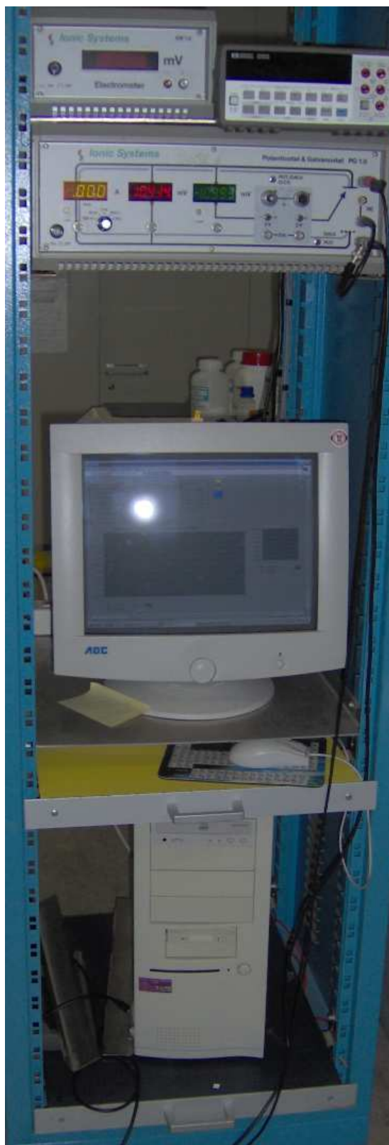
Fig.3.3 A photographic representation of the Galvanostatic/potentiostatic full measurement setups with the computer and potentiostat. The sample was kept in the Kiel-Cell where it was also used for measurements at different temperatures of the cell.
