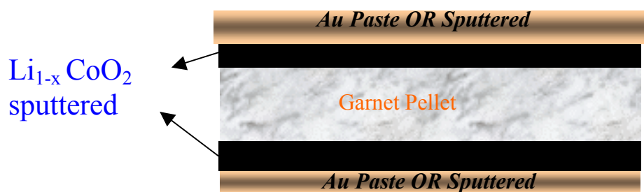
Fig. 5.24 Schematic representation of the supercapacitor assembled from Garnet pellet as electrolyte, Sputtered \text{LiCoO}_2 as electrode on both sides, and Au paste Or Au sputtered film as a current collector.
