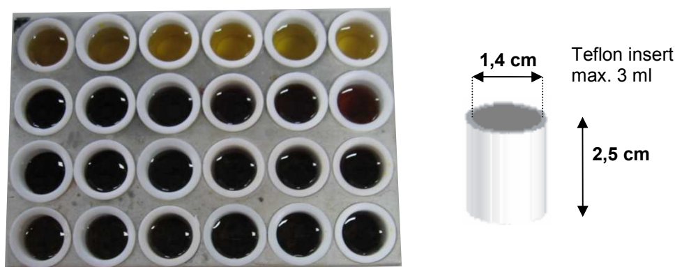
Figure S1 24-High-throughput reaction block (left) and the corresponding teflon insert (right) with a maximum volume of 3 ml.
