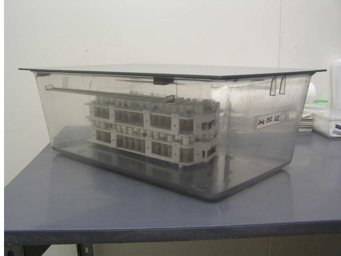
Fig. 14: Transparent box (Makrolon cage) as it was used for storing the experimental racks in the incubator or climate chamber, respectively.
