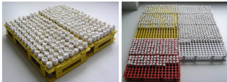
Fig. 13: Most of the experiments were carried out in lidless 2.2ml experimental tubes covered with dental rolls. The experimental tubes were stacked in racks.
