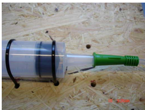
Photo 3. 4 mm junction between syringe and suction/irrigation conduit
