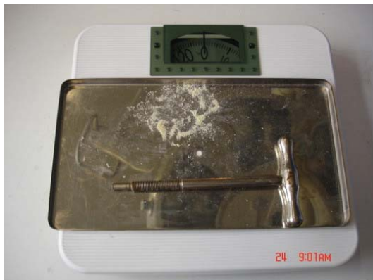
Photo 10. Instruments for manually crushing debris and measuring crushing force.
