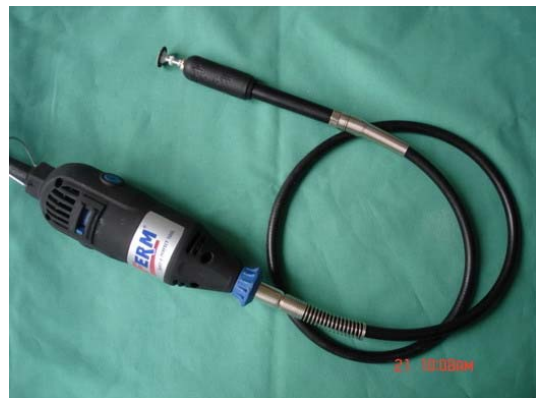
Photo 11. Electric cutter applied to derive calcium of surrounding valve tissue
