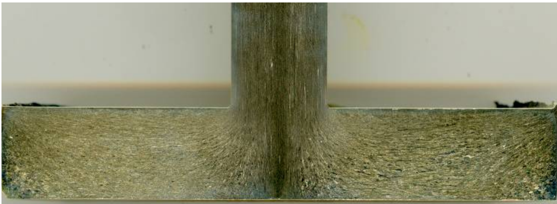
Figure 8.5: Longitudinal section of the extrusion remainder (ZE10) at ram speed of 5 mm/s
