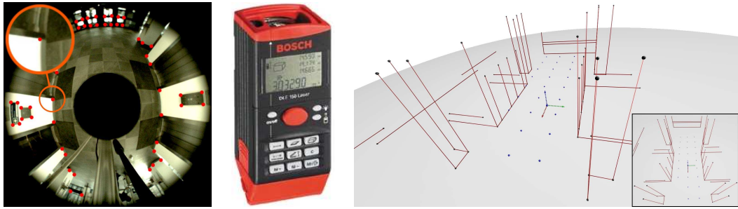
Fig. 8.10: The 3D-line model (right) of the entrance hall was built from point measurements (red dots, left) using a laser device. The blue dots in the right image indicate the 25 sensor positions.
