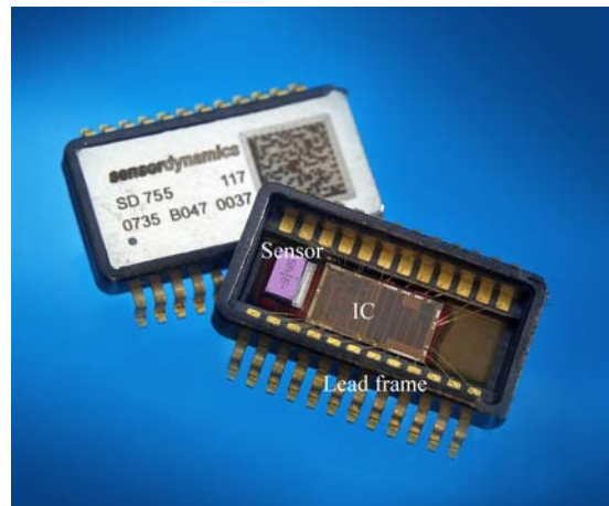
Figure 1.3: MEMS package of an inertial measurement unit (Source: SensorDynamics).
