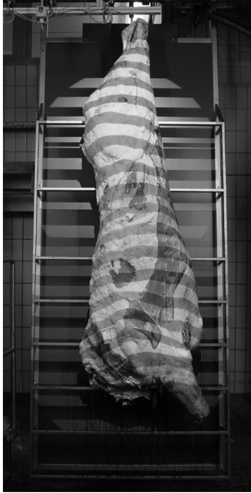
Figure 1: Video image of a carcass. The bending of light stripes is used to cover information on color and conformation (picture provided by E+V Technology GmbH, 16515 Oranienburg, Germany).
