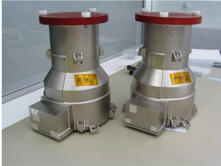
Figure 1.2: The finished RAD sensor heads placed on a clean-room bench. The label FM1 denotes the flight-spare whereas FM2 marks the actual instrument that will be landed on Mars. The sensor heads will be attached to the RAD electronics boxes (not shown here) with their feet. The scale of the instruments in the picture is about 0.5\times . The red items on top of the instruments are protective covers that will be removed before flight.
