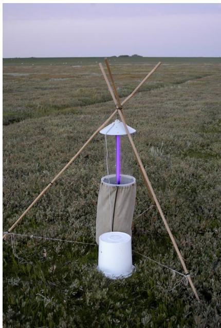
Fig. 3.1: Light trap with super actinic fluorescent tube.
