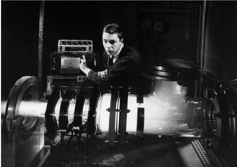
Figure 1.3: Gas discharge being operated by Raymond W. Plamer at the Lewis Electromagnetic Propulsion Division, Cleveland, Ohio 1961. Photograph downloaded from [37].
