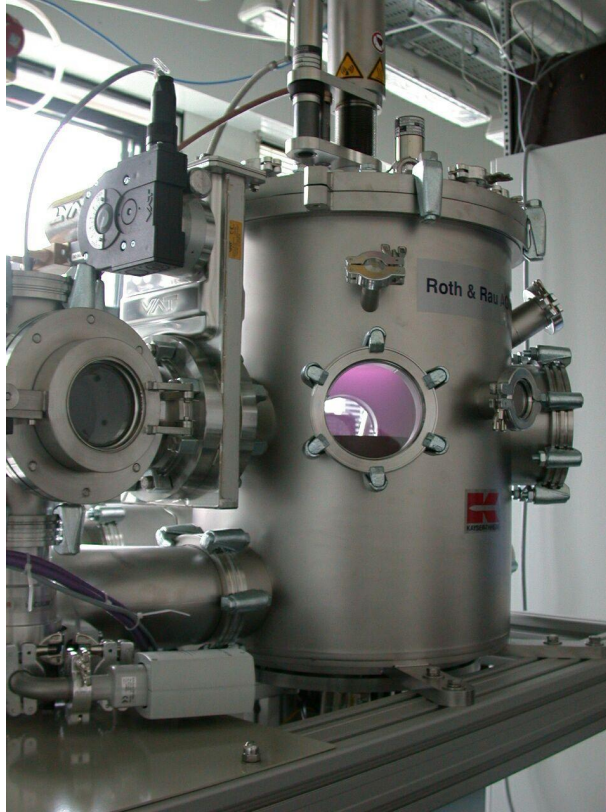
(a) PULVA-INP in action. Inside the window, an argon plasma (pink) can be seen.
