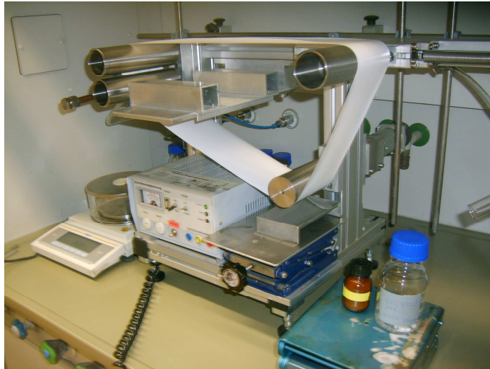
Figure 6.3: Dip-coating equipment, coating stage.
