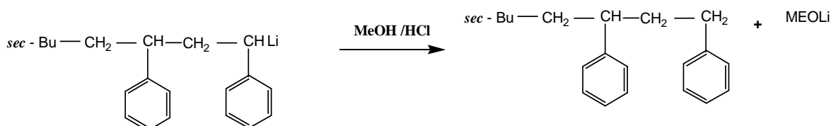
Figure 2.2: Synthesis of polystyrene via anionic polymerization.
