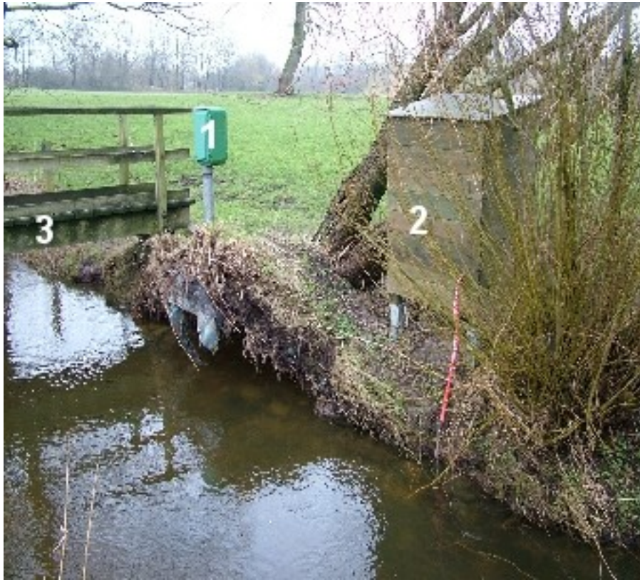
Fig. 17: Sampling point at the Kielstau with water level recorder (1) and automatic sampler (2). (3) indicates position underneath bridge of flow meter in the Kielstau.
