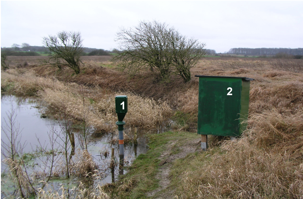
Fig. 16: Sampling point Moorau with mechanical water level recorder (1) and automatic sampler (2).
