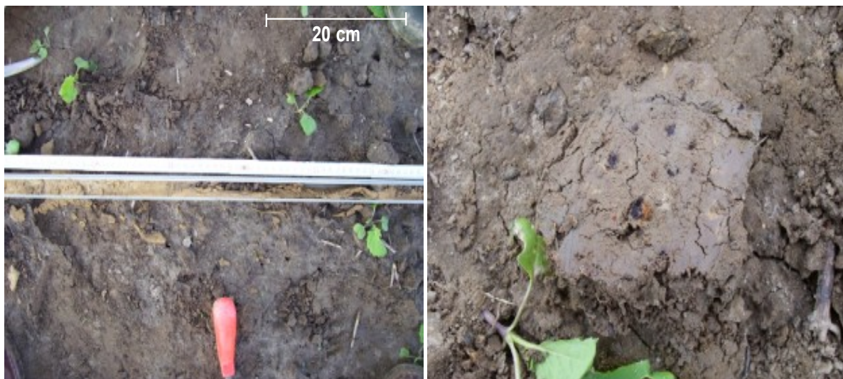
Fig. 35: Soil type determination with soil drill (l) and stagnant moisture characteristics in the subsoil (r)
