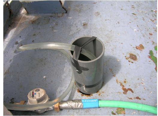
Fig. D. Pump sampling contrivance with water meter and 63µm sieve built during MARSUED IV in January 2008.
