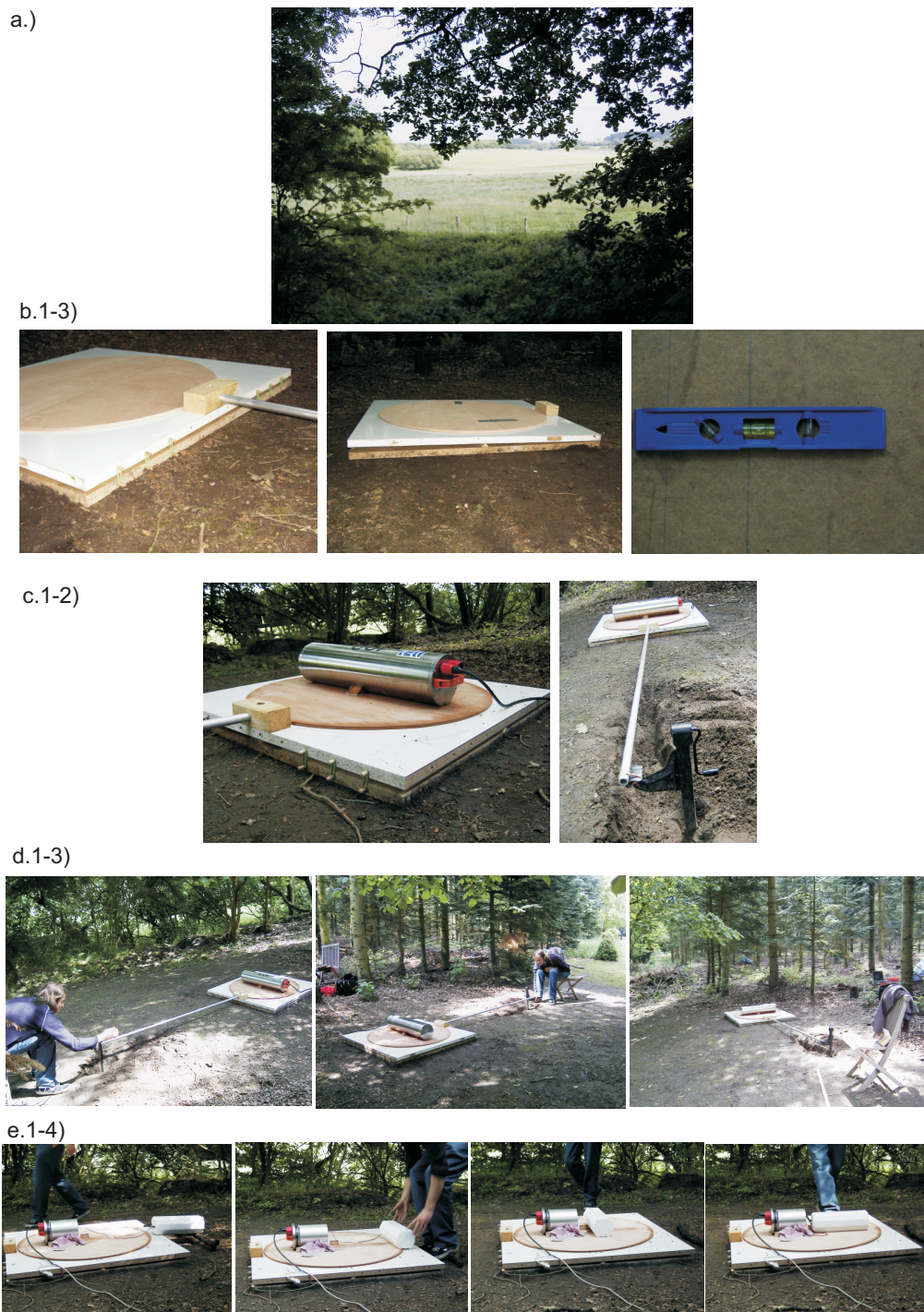
Figure 7.22: Pictures of Shaking Apparatus and test measurements at Viehdamm, apparatus was designed and build by Björn Lewitz.
